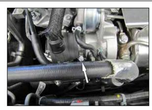
5. Install the provided coupler (5-1045) onto the turbo inlet and secure with the provided hose clamp.
