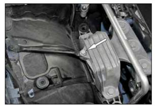
9. Remove the bolt shown from the fender brace. NOTE: This bolt will be reused in the next step.
