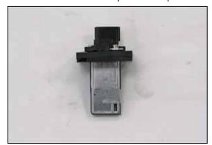
11. Remove the mass air sensor from the factory air filter housing. Install the sensor and provided gasket onto the K&N® filter adapter as shown.
