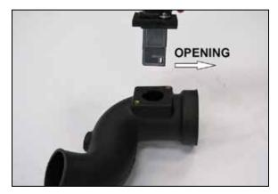
12. Install the mass air sensor assembly into the K&N® intake tube and secure with the provided
