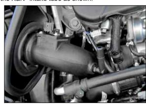
14. Install the K&N® intake tube assembly through the heat shield and then into the coupler on the turbo. Adjust the tube and heat shield for best fit and then secure the hose clamp and heat shield
